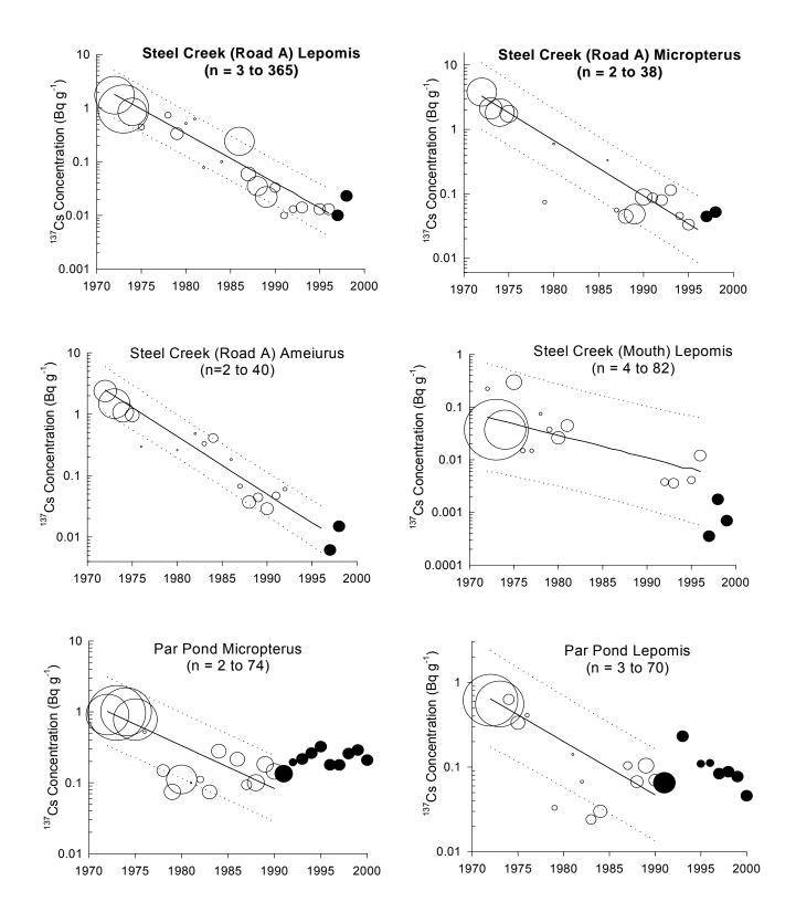
Figure 1. Changes in <sup>137</sup>Cs in whole fish regressed against time for fishes at the Savannah River Site. Circles represent data used to compute <sup>137</sup>Cs half-lives ( $T_e$ 's). Solid circles represent data collected from 1997-2001. Symbol areas are proportional to the number of fish in each sample. Solid lines represent regression lines; dotted lines represent 95% prediction intervals. Statistical parameters for the regression lines appear in Table 1.
